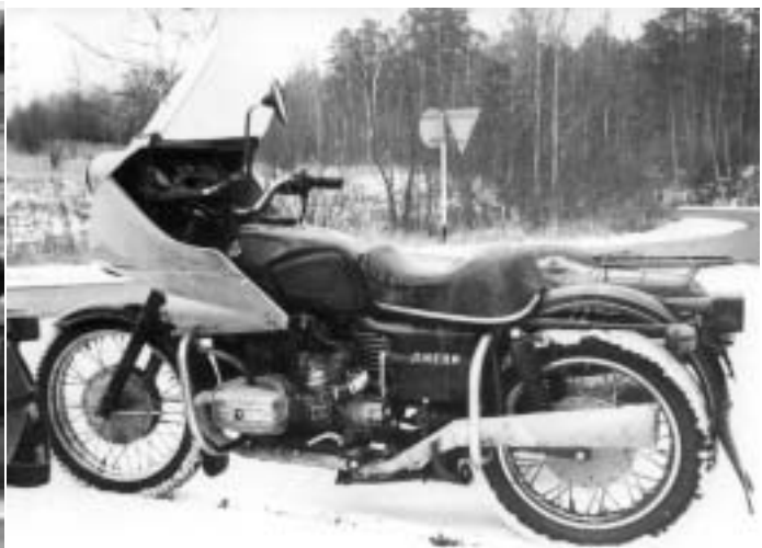
Left and Above – Kiev ‘Escort’ motorcycle, note the single big seat, and the protection bars. Photos from JRamba.
