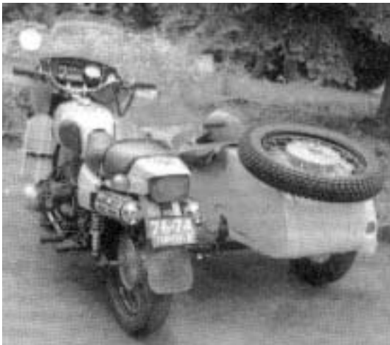
Dnieper, note high level silencer Photo JRamba
