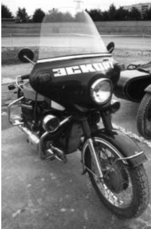
Left and Above – Kiev ‘Escort’ motorcycle, note the single big seat, and the protection bars. Photos from JRamba.
