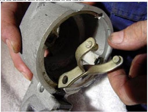
Step # 7 When you remove the actuator arm, note that two sides of the arm are different. One side is curved, the other side is flat.
