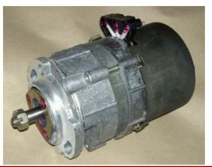
The higher-output capability of the 14.3771 alternator was needed to provide a migratory path for electric-start, in an urban (slow-speed & traffic lights) driving environment.
