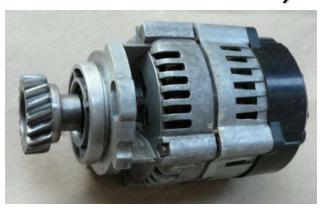
The 14.3771, 12-Volt alternator (affectionately known as the RPOC) developed a bad reputation for exploding and often taking the engine with it, hence the term "Russian hand-grenade".
