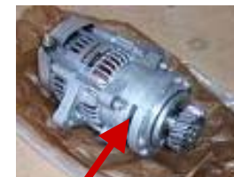
100211-1680 Alternator “+” Cush Adapter and Pinion Gear
