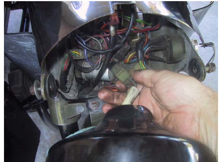
Pull the Molex connector for the head light apart.
