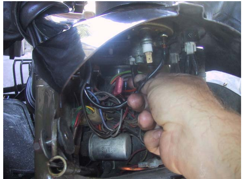
Pull the rear illumination bulb free.
