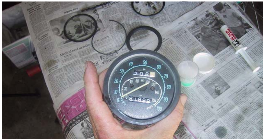
Drop the speedo mechanism into the can...
