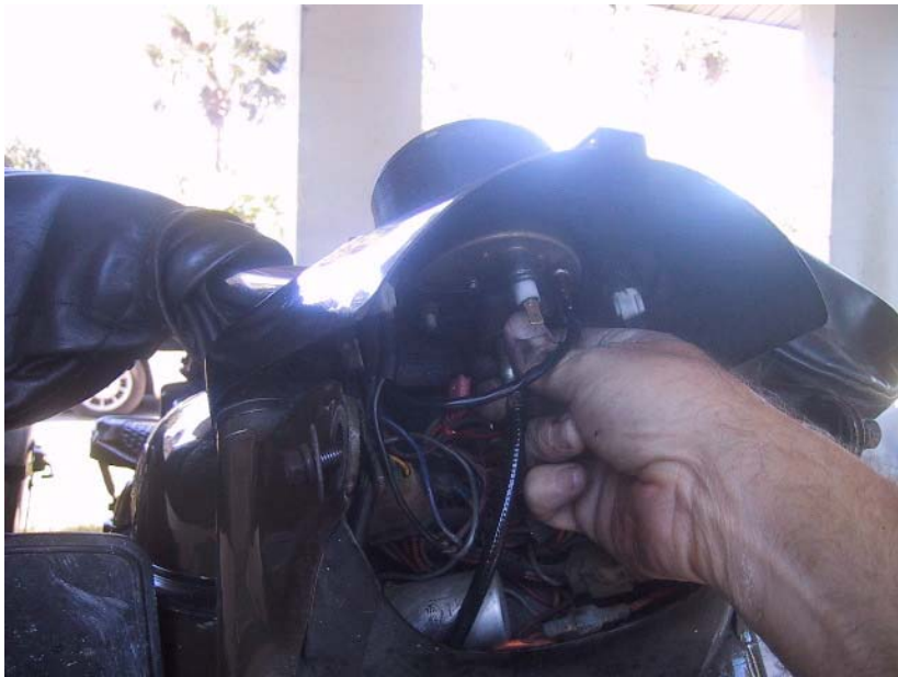
Unscrew the speedo cable and pull it free.
