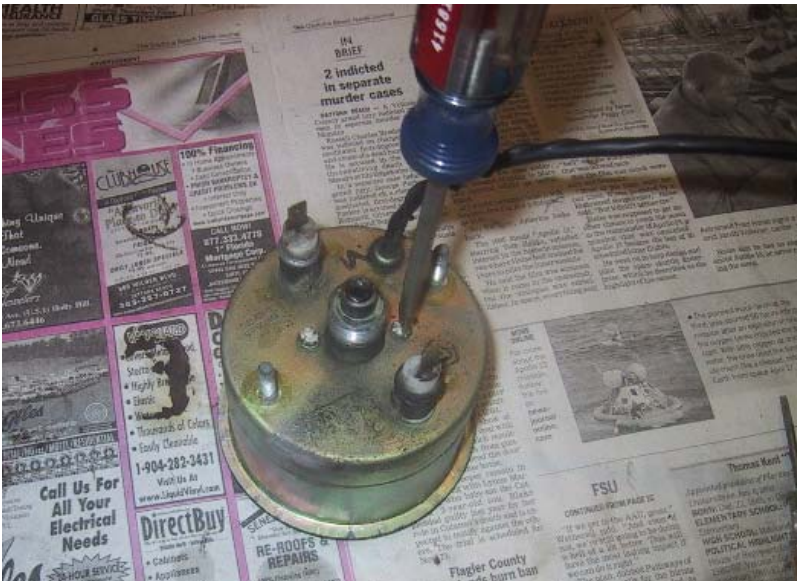
Use a flat blade screwdriver to remove the two screws that hold the speed in the body can.
