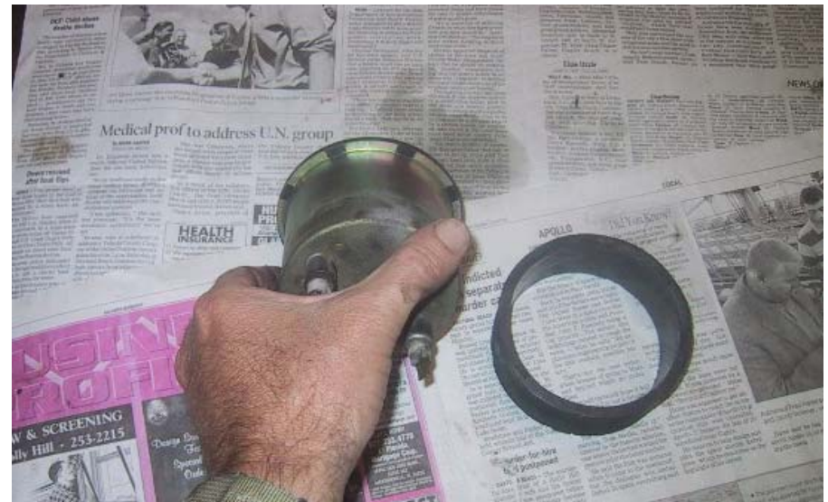
Here you can see a few of the tabs that hold the metal face plate ring on. We'll get to these later.
