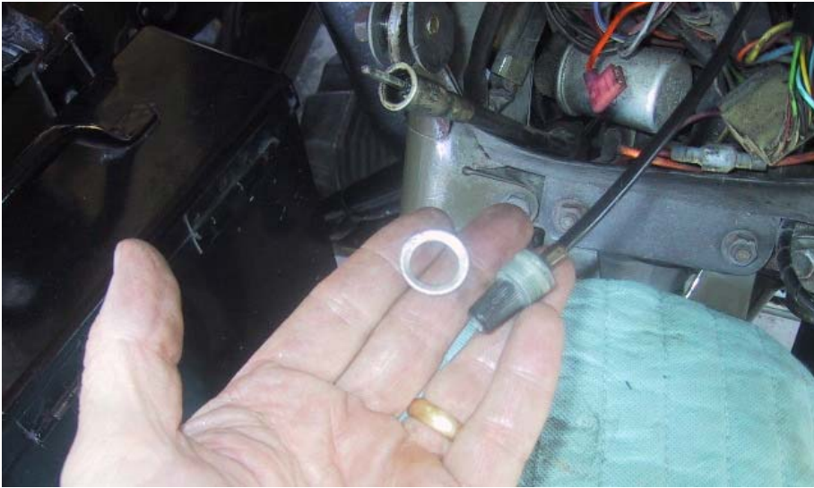
...be watching for the spacer ring that is under sheet metal at the base of the trip meter knob...it can disappear into the "rats nest".
