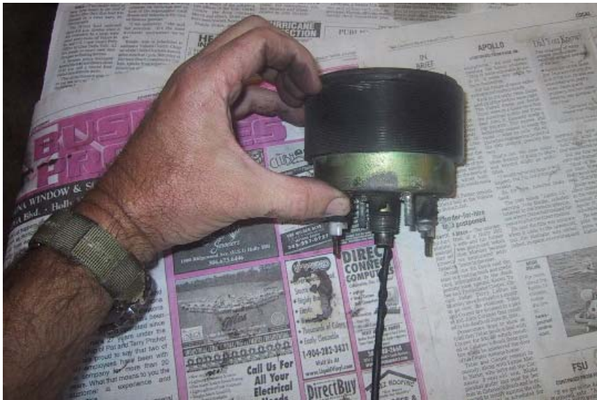
First step in disassembling is to remove the protective rubber...use your finger tips on each side...
