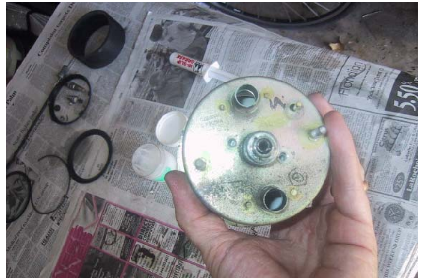
...and make sure the rubber seal holes line up.
