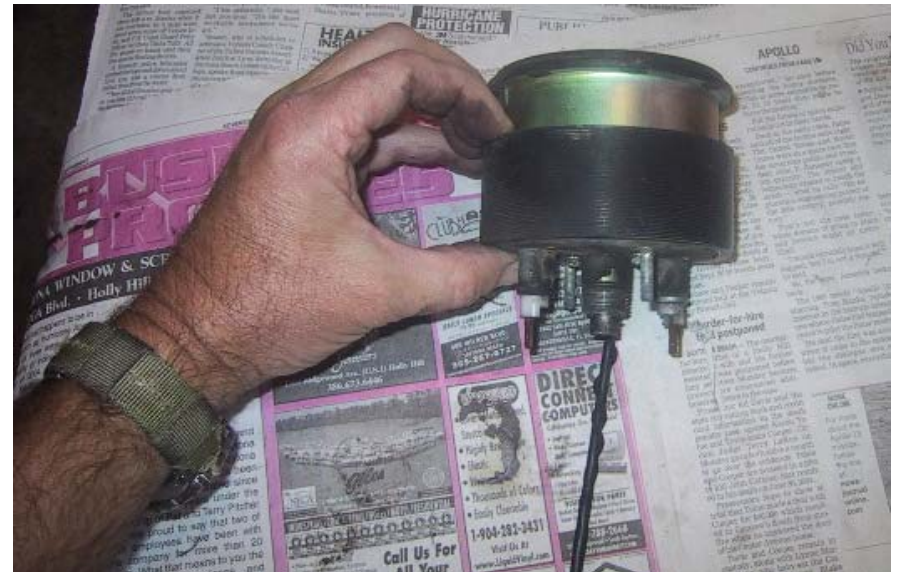
...and pull down. A squirt or two of silicone spray may be helpful.
