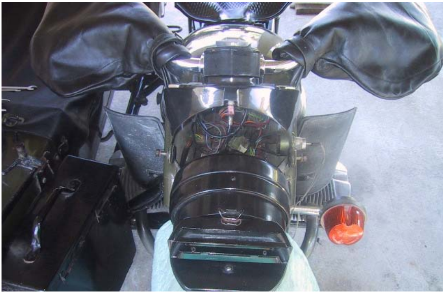
remove the head light assembly without removing the bolts.
