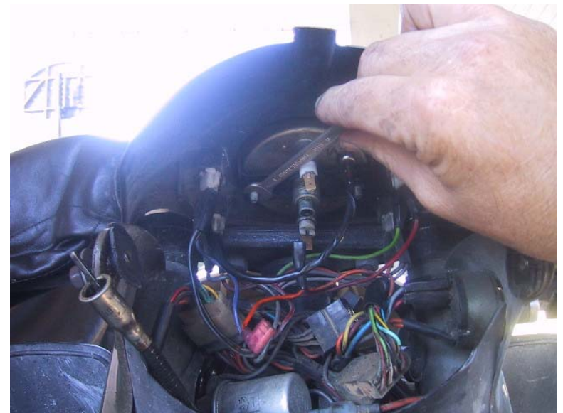
Use the 6mm wrench to remove the nuts/washers securing the bar to the speedo. Careful not to drop the nuts, they are tiny!
