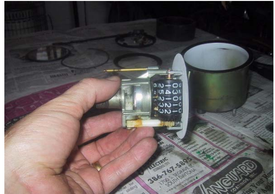
...and yet another, this time the top showing the trip meter Geneva mechanism.
