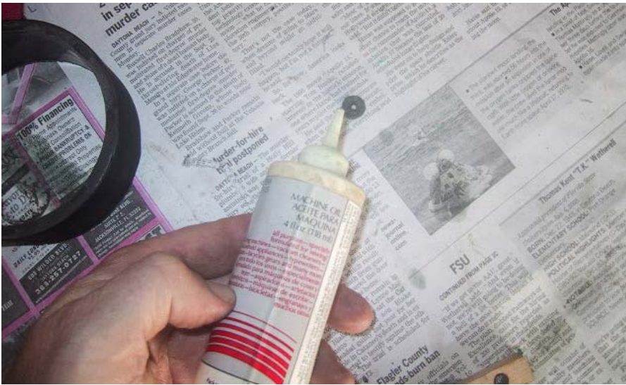
Put a drop or two of machine oil on the felt dirt washer for the odometer cable...
