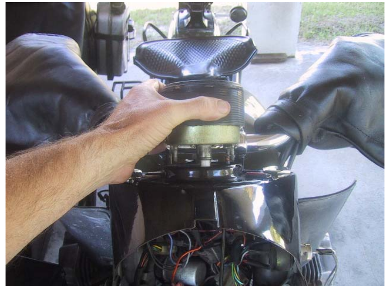
You can now lift the speedo free of the dash.
