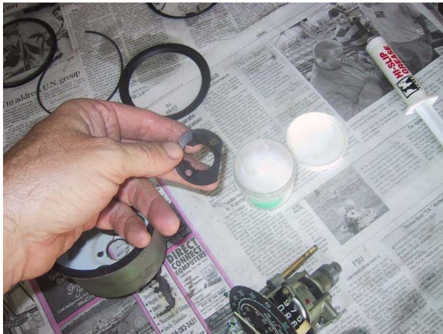
Silicone grease on both side of the can seal...
