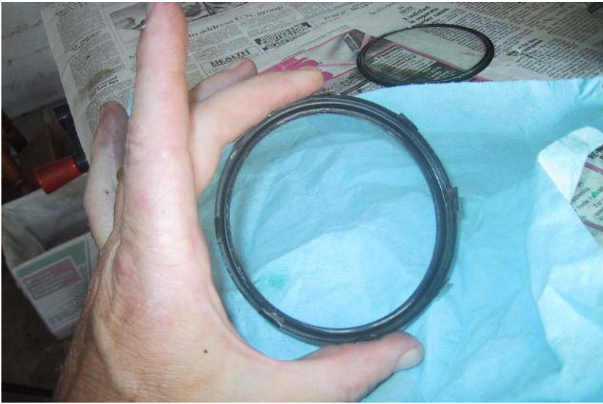
The thin rubber O-ring goes inside the metal ring with the tabs. Use four dollops of silicone grease to hold the O-ring in place.
