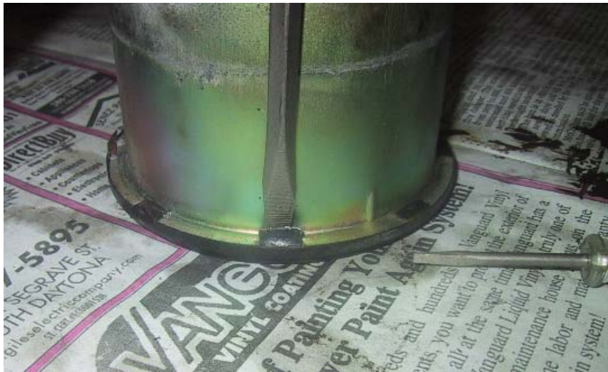
...bend the face plate ring tabs up.
