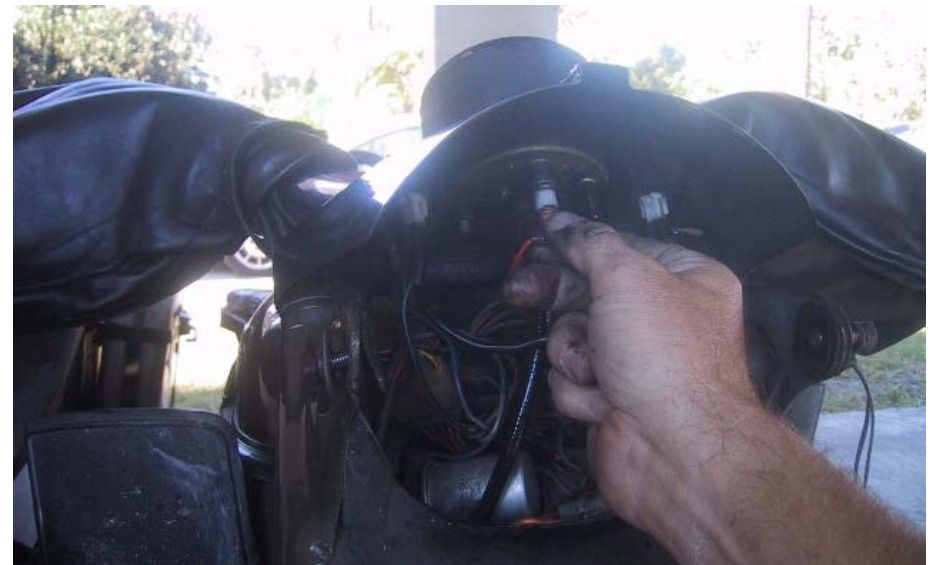
Pull the front speedo illumination bulb out. The connector/bulb is a press fit into the speedo housing.
