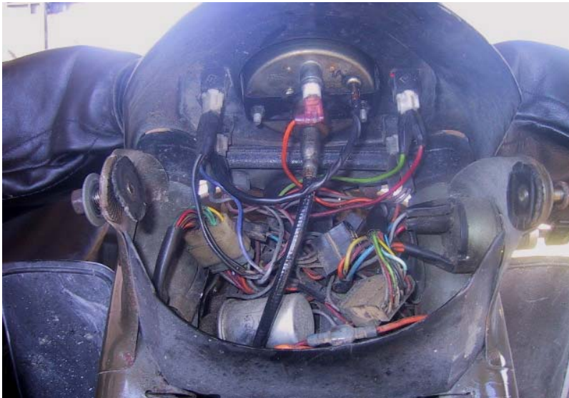
This is a good time to clean and grease all the fuses and connections in the "rats nest".
