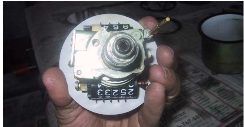
A few drops of machine oil need to be put between the speedo cable drive socket and the threaded collar. Not down the hole in the middle!
