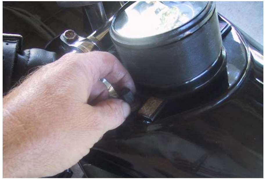
If you have a trip meter, you'll need to remove the lock ring at the knob...
