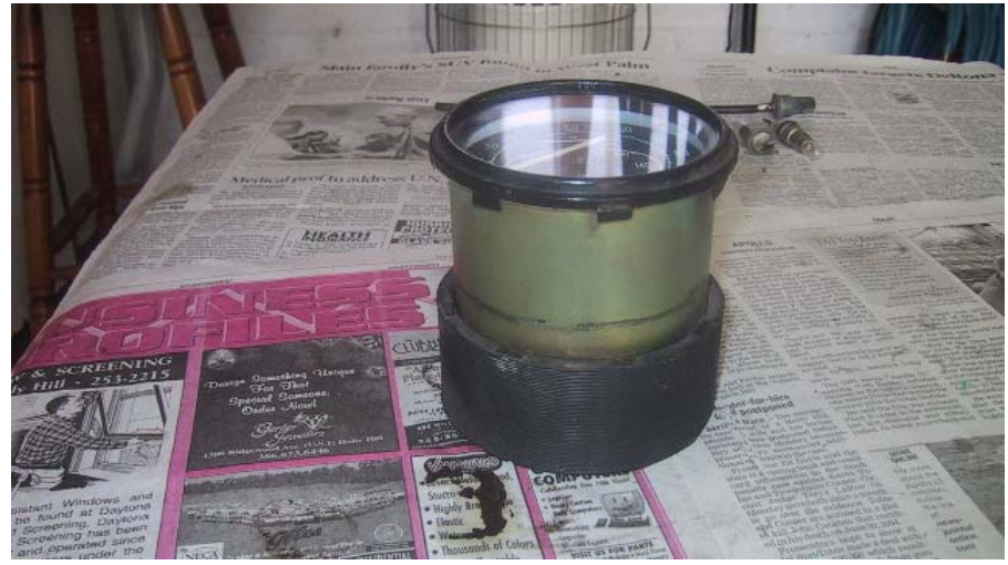
Set the speedo can in the rubber protective ring as a stand. Put the metal ring on and bend the tabs in a bit to hold it in place.
