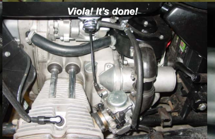
Be sure to cap vacuum line port on top of left side carburetor!
