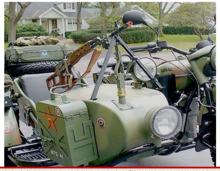
Russian bikes can either use the front-mount to hold the straight pintle (shown above) or the "T" pintle shown later.
