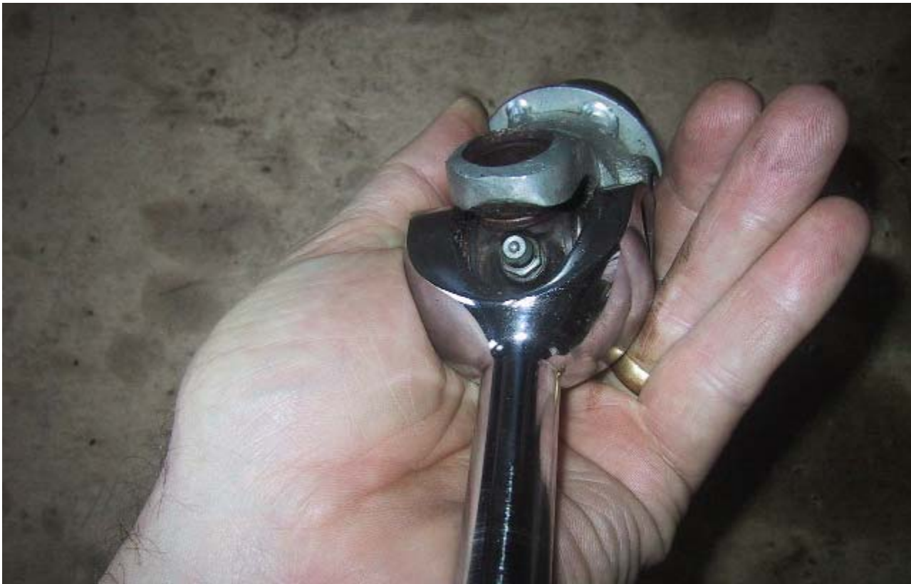
If the U-joint has a grease zerk fitted, it is a good idea to remove it before disassembling to prevent damage. Especially if you are just servicing or re-using the U-joint.
