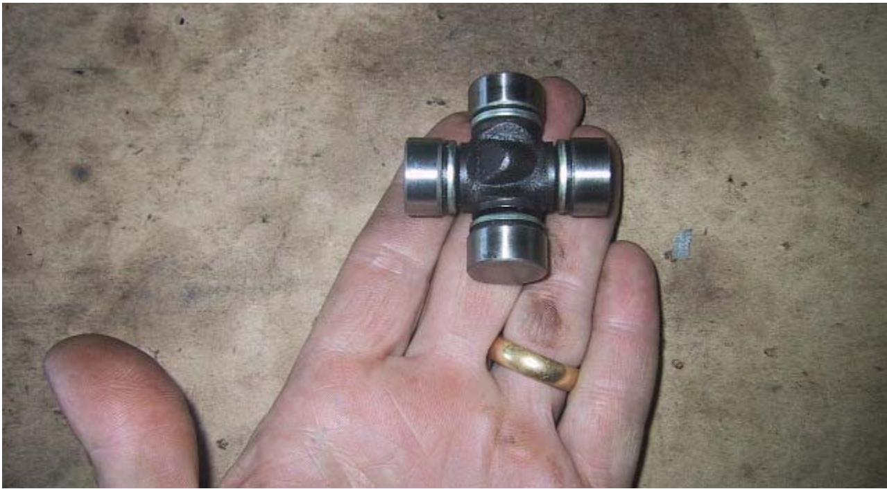
The new U-joint assembled. The cross is the center part, with a metal cup hold a rubber grommet followed by the outer races holding 18 needle bearings each.
