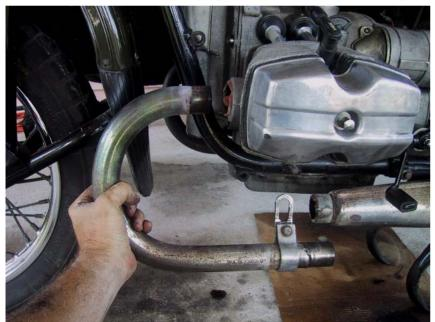
Slide the header pipe free of the mounting clamp and set aside where it will not get damaged or stepped on.
