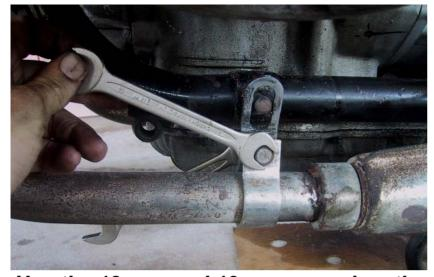
Use the 12 mm and 13 mm wrenches the loosen the header pipe mounting clamp.
