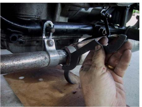
...to loosen the header/muffler collar nut. It does not come off the muffler; it just needs to be loosened.
