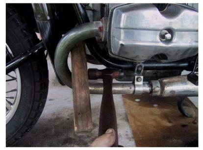
Use a dead blow hammer or block of wood and hammer to knock the header pipe free of the cylinder head and muffler.
