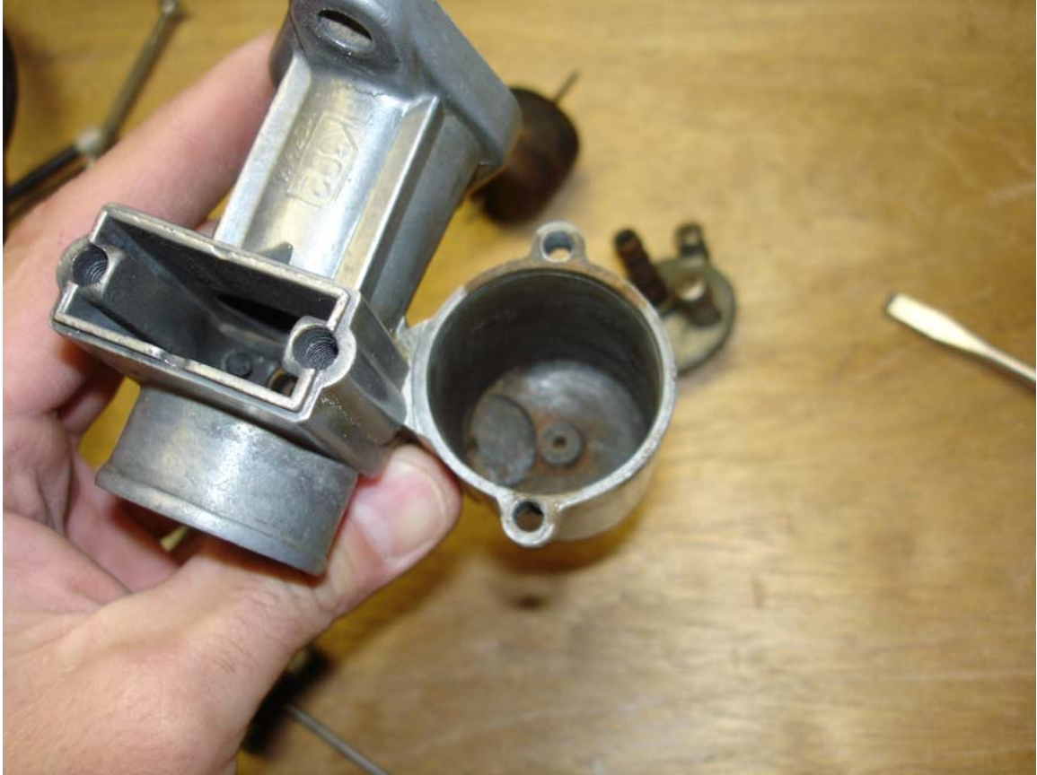
This is the float guide which can contain buildup, hindering the actuation of the float.
