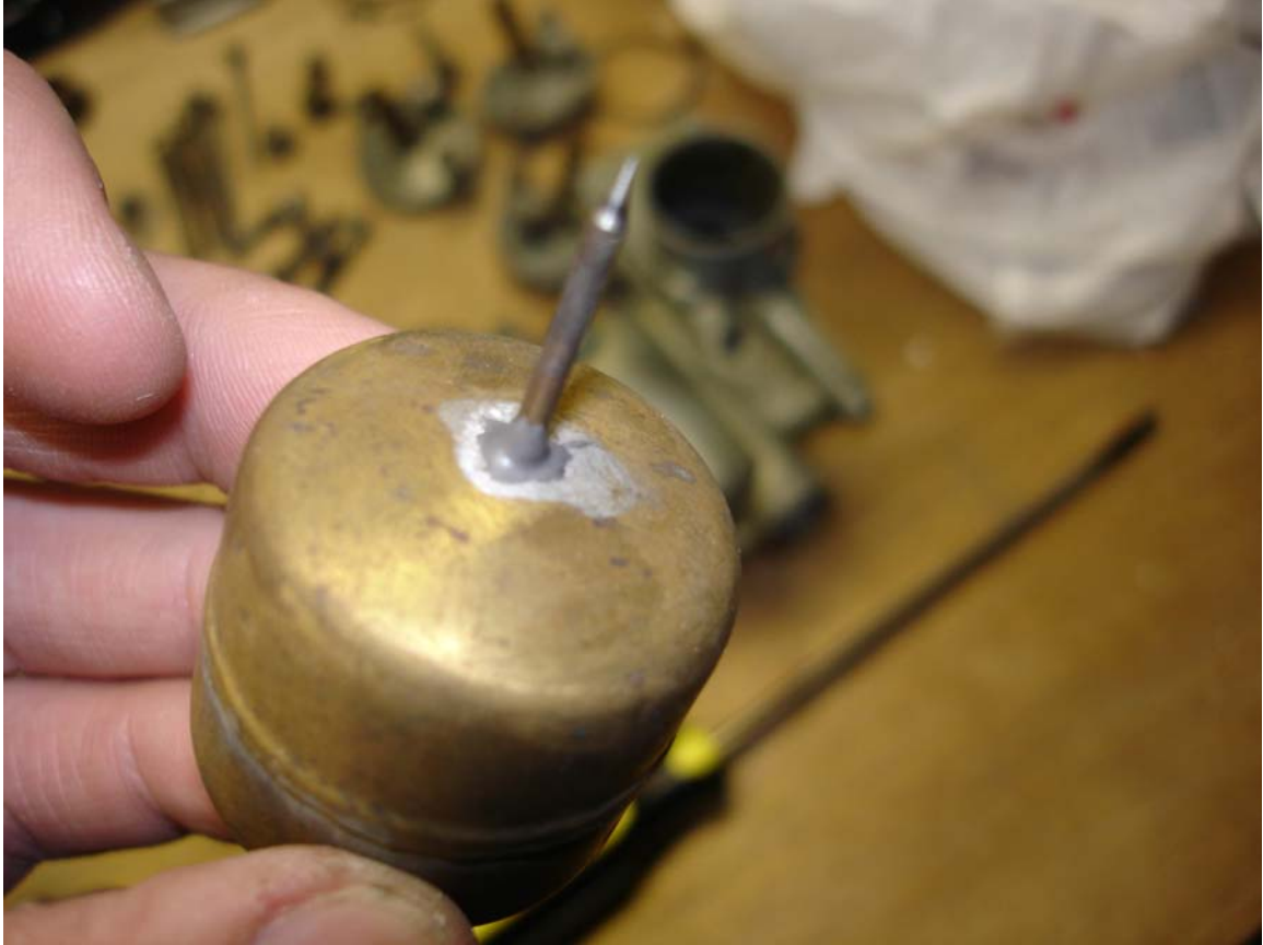
Float sealed with light application of JB Weld.
