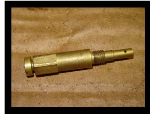
Here it is with a jet screwed in. Note there's no fiber washer, something you'd definitely not want to forget when you put your carb back together.
