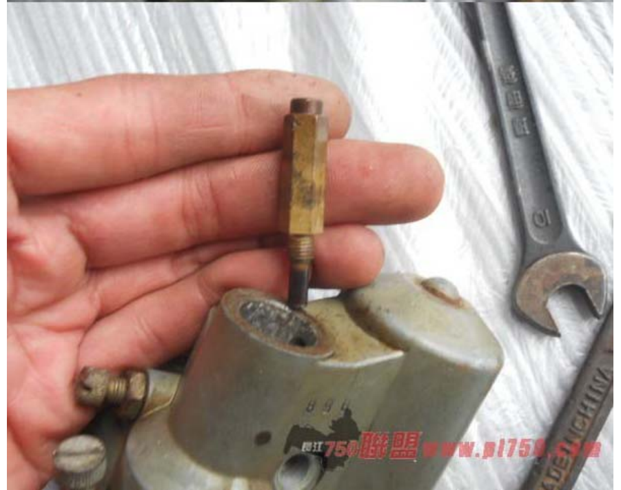
Remove and clean the main jet assembly.
