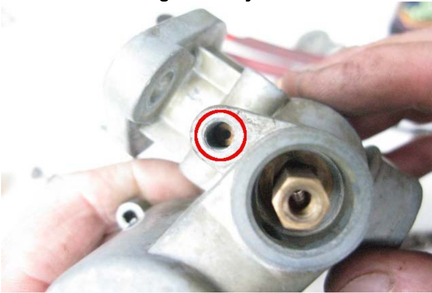
Looking into the idle jet hole, you can see the idle jet. The black 1.5 mm hole in the center of the brass is NOT the idle jet, just the base of it. The actual orifice of the idle jet is 0.010" or so.
