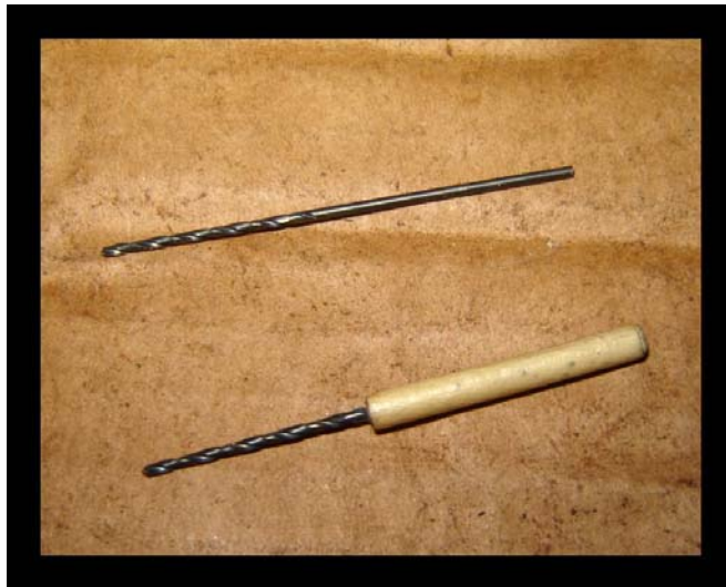
These are #57 bits (1.0922mm.) Unfortunately, that's too small for the Dremel's chuck so I wrapped it with masking tape to increase its diameter.
