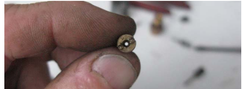
The main jet orifice. The main jet is a restriction located below the needle valve that limits the amount of fuel that can be drawn through needle valve at full throttle or near full throttle operation. It really doesn't do a lot most of the time. If you plan on testing your main jet by the color of your plugs, remember to color the plugs under full throttle.
