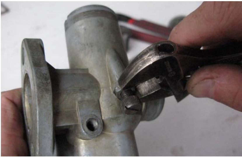
Loosening the idle speed screw (throttle slide stop screw) lock-nut.
