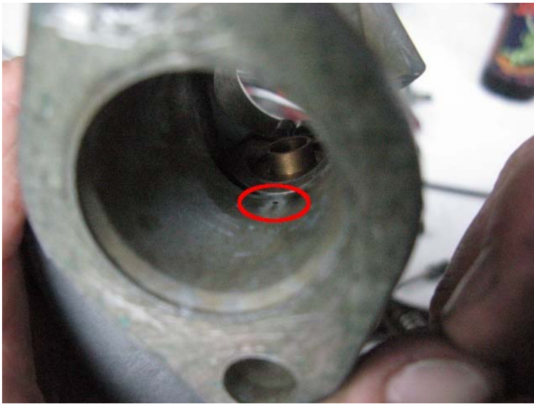
This is the idle mixture hole visible at the bottom of the carb bore on the engine side of the throttle slide.
