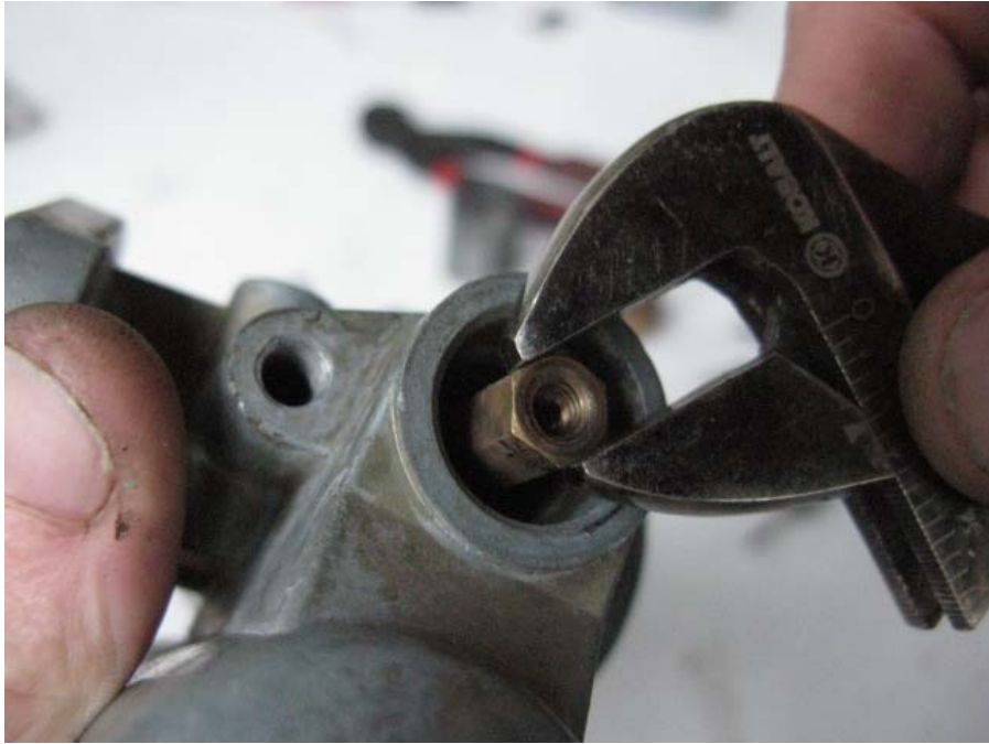
Removing the needle valve venturi tube.
