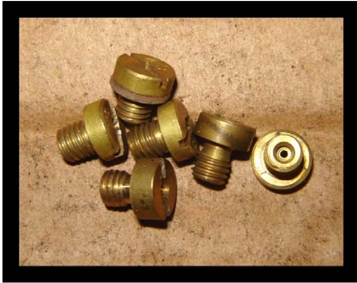
Look at all these jets! I harvested them from some junk carbs I had laying around.
