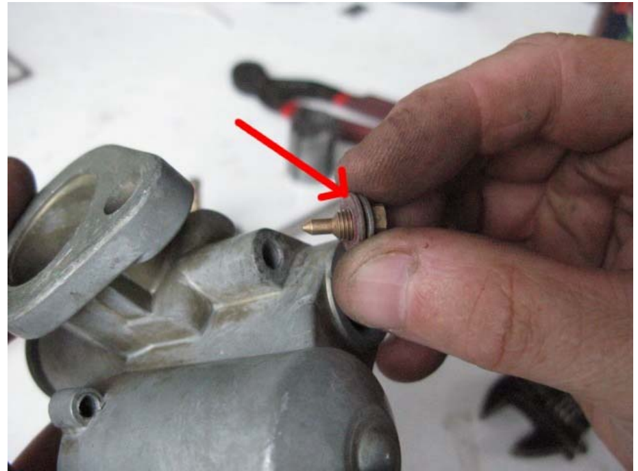
The idle jet cover, note the washer. This is not an adjustable screw. You just screw it all the way in. The taper at the tip works in conjunction with a tiny idle jet to mix the air and gas in the idle mixture.
