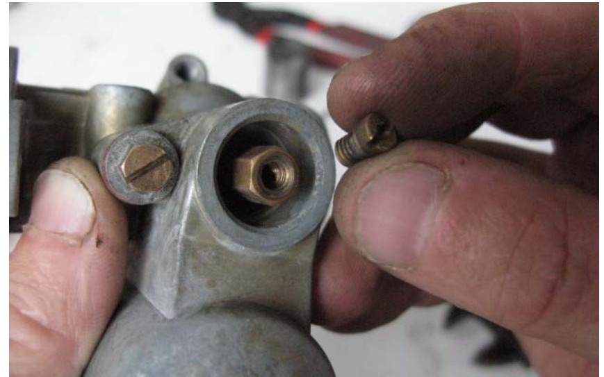
The main jet exposed for inspection and cleaning.
