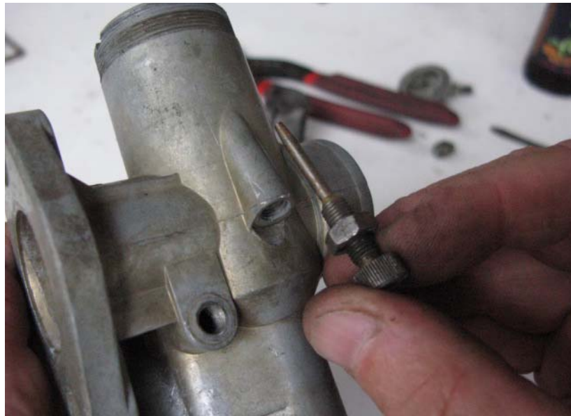
This is the idle speed adjustment. Screwing in will lift the main jet needle, and increase the idling speed. The idle speed screw out for inspection. Tightening it in raises the throttle slide increasing the idle speed.
