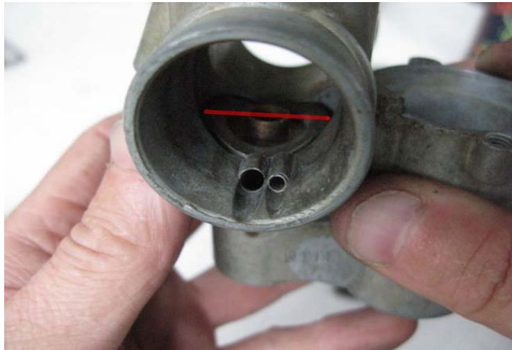
The small hole on the left is the idle air inlet.
