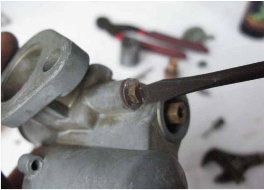
Removing the idle jet cover.
