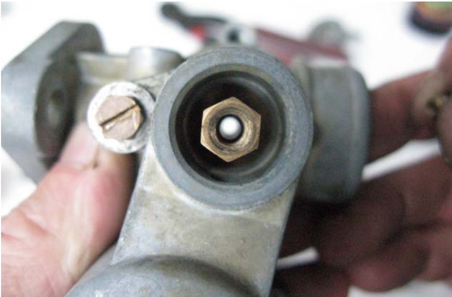
This is a shot of the needle valve bore from the bottom of the carb. It should be clear.
