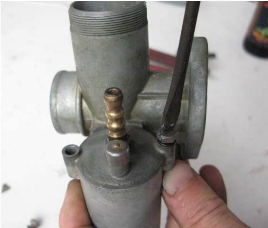
Removing the float bowl cover.
