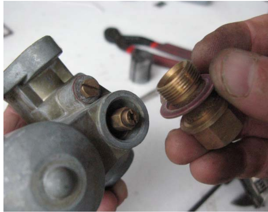
The fuel well should have a fine screen wrapped around the outside and a washer to seal it to the carb body.
