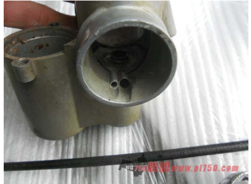
This is the idle mixture hole visible at the bottom of the carb bore on the engine side of the throttle slide.
