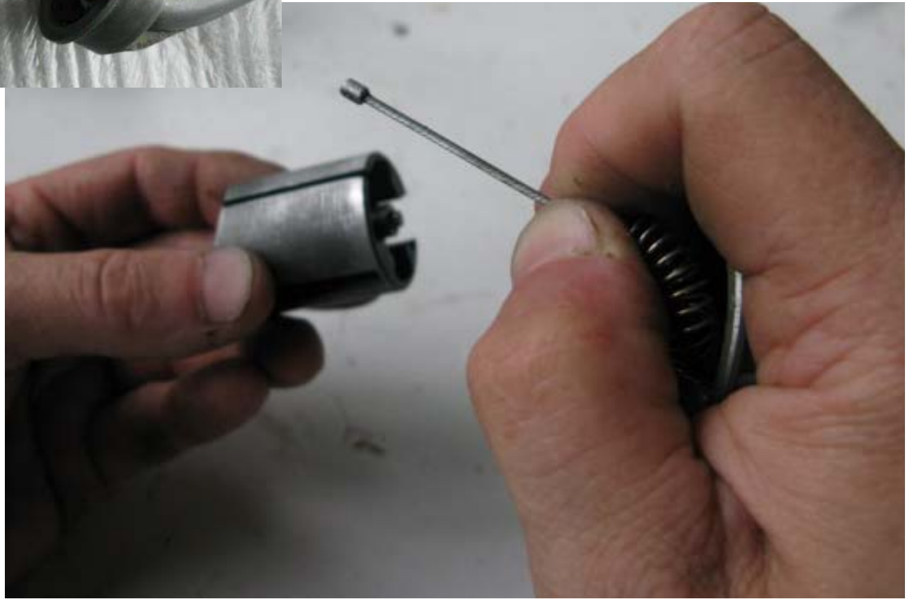
The cable and spring held in position for reinstallation.
