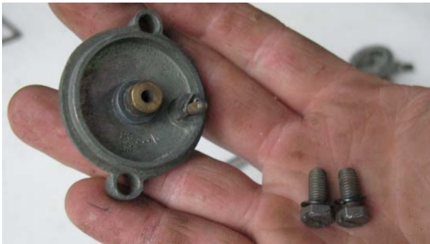
The two screws should have lock-washers.
