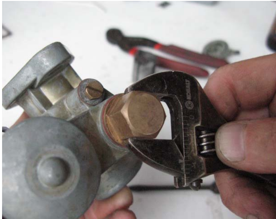
Loosening the main jet fuel well.
