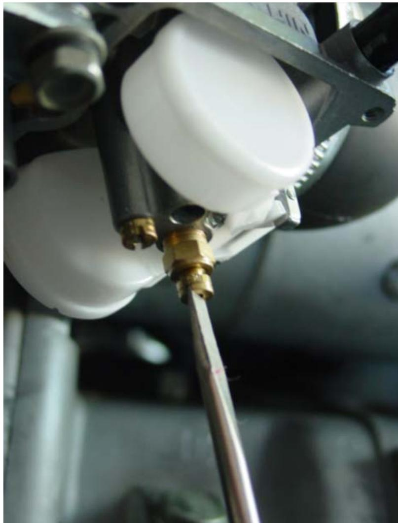
***Remove and replace the main jet using a proper screwdriver.***
