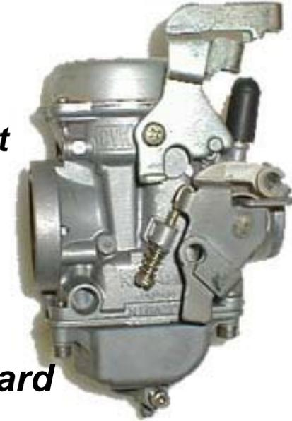
**The Keihin carburetor was fitted to pass stringent emission regulations (EPA).**
