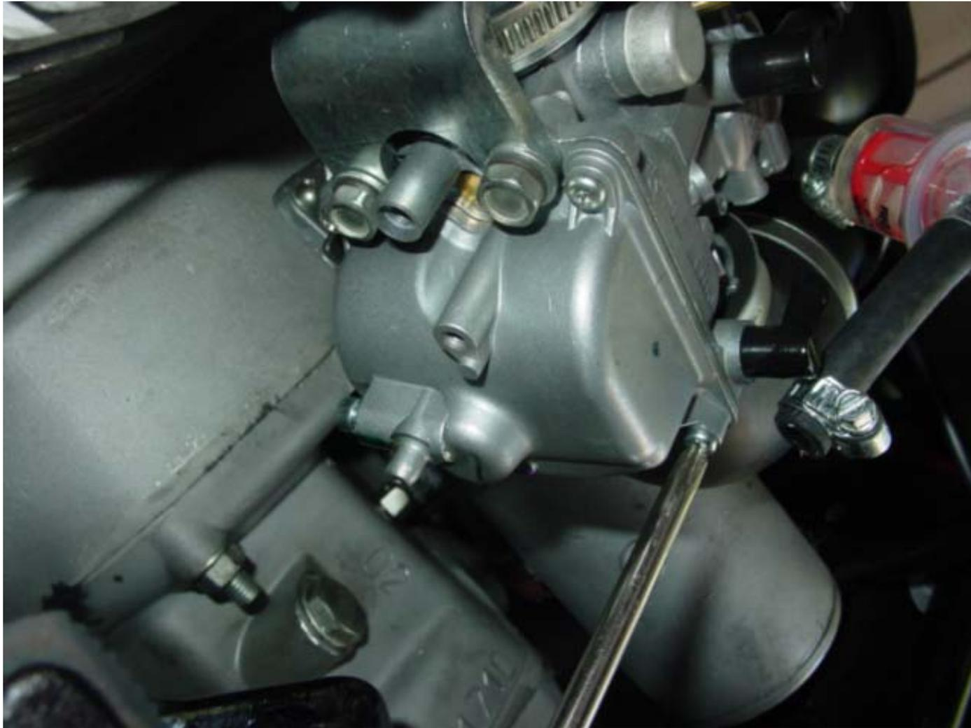
***Use the proper screwdriver to remove float bowl screws.***
