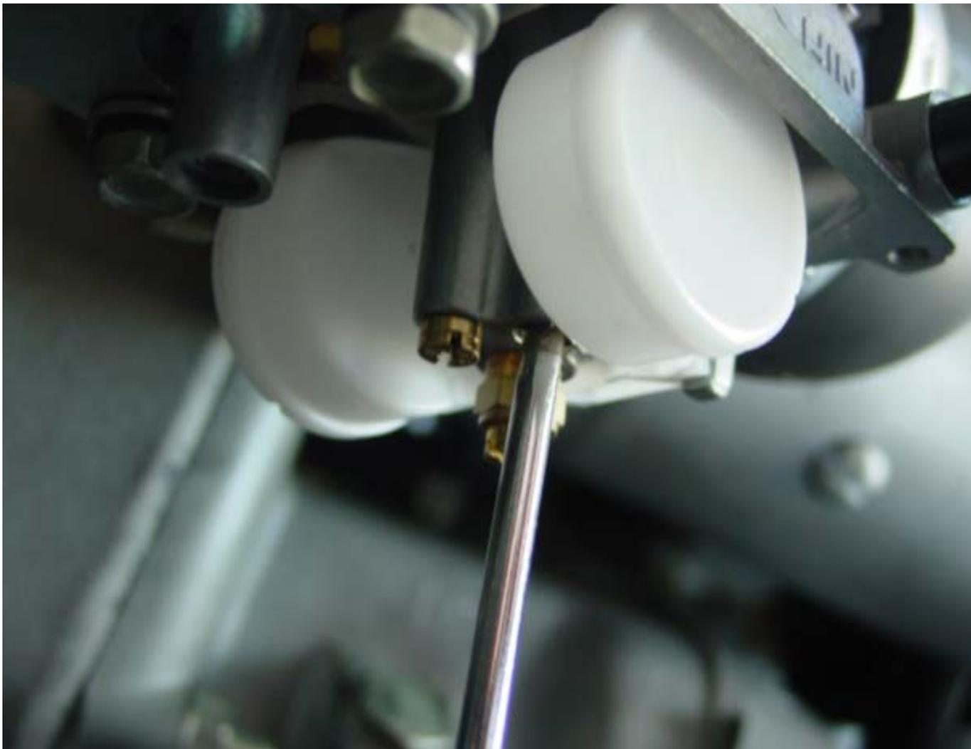
***Remove and replace the pilot jet (recessed).***
