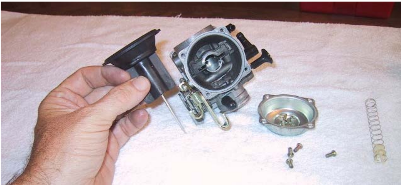
...and the diaphragm/slide and needle.
