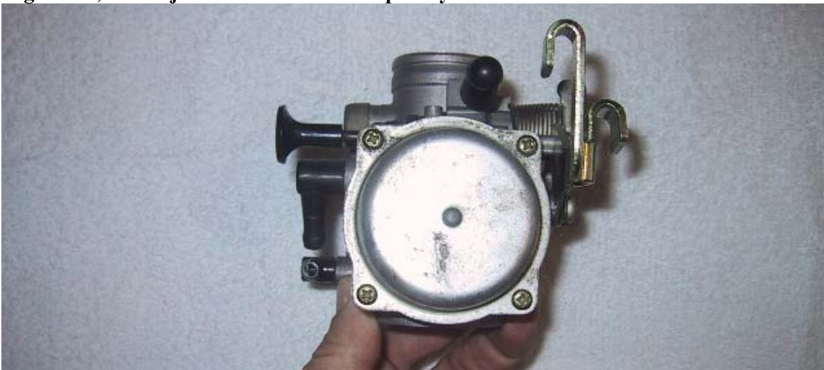
Top view looking at diaphragm cap.
