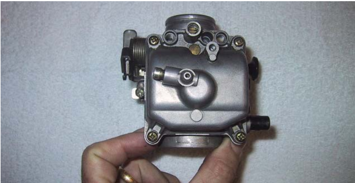
Bottom view looking at carb bowl drain.
