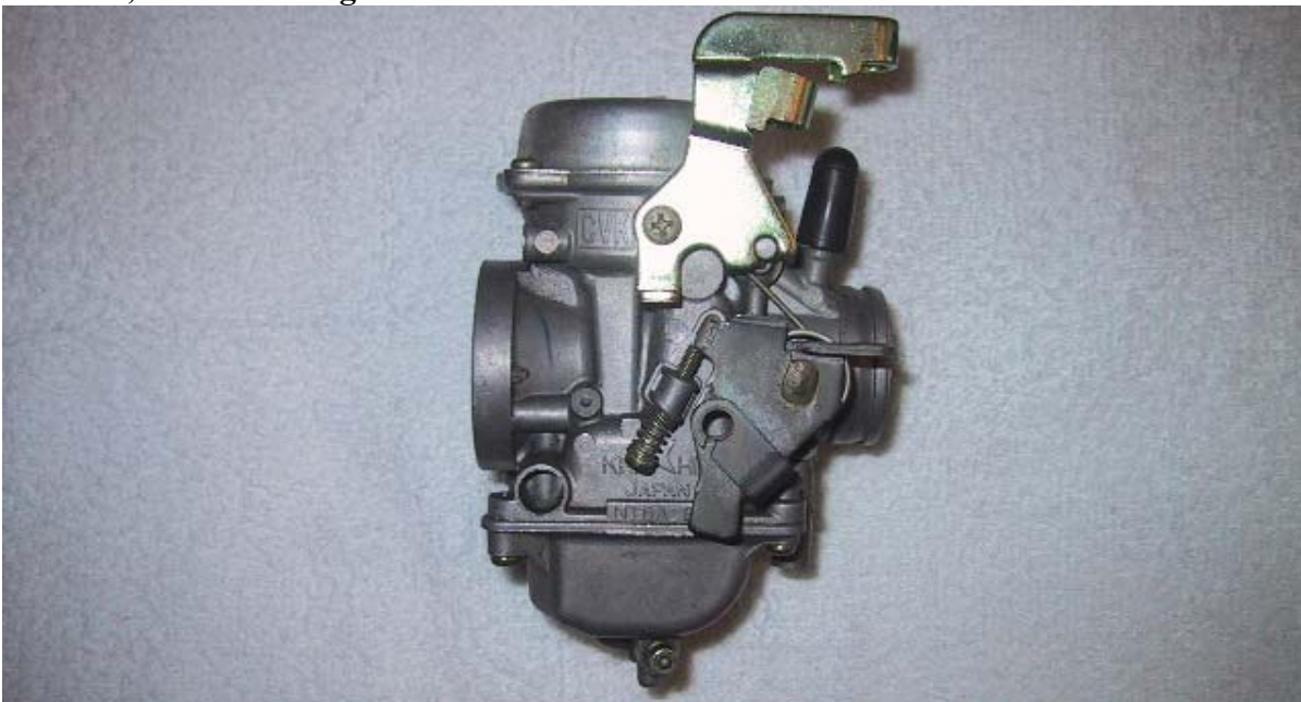
Right side, idle adjustment screw can be plainly seen.
