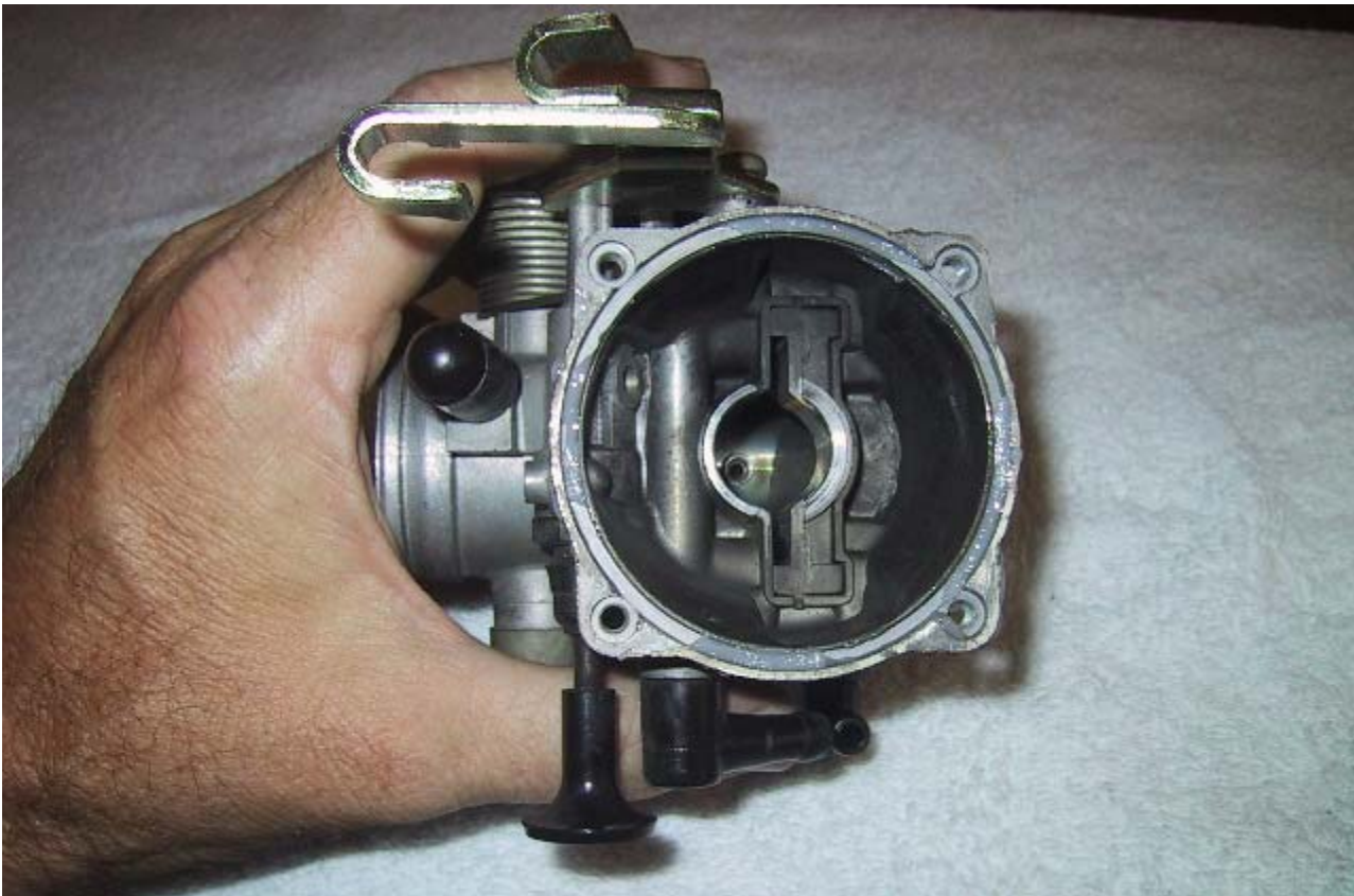
Keeping the diaphragm from popping out of the groove can be a challenge...especially if doing this on the bike. A little silicone grease in the groove helps hold the diaphragm down.
