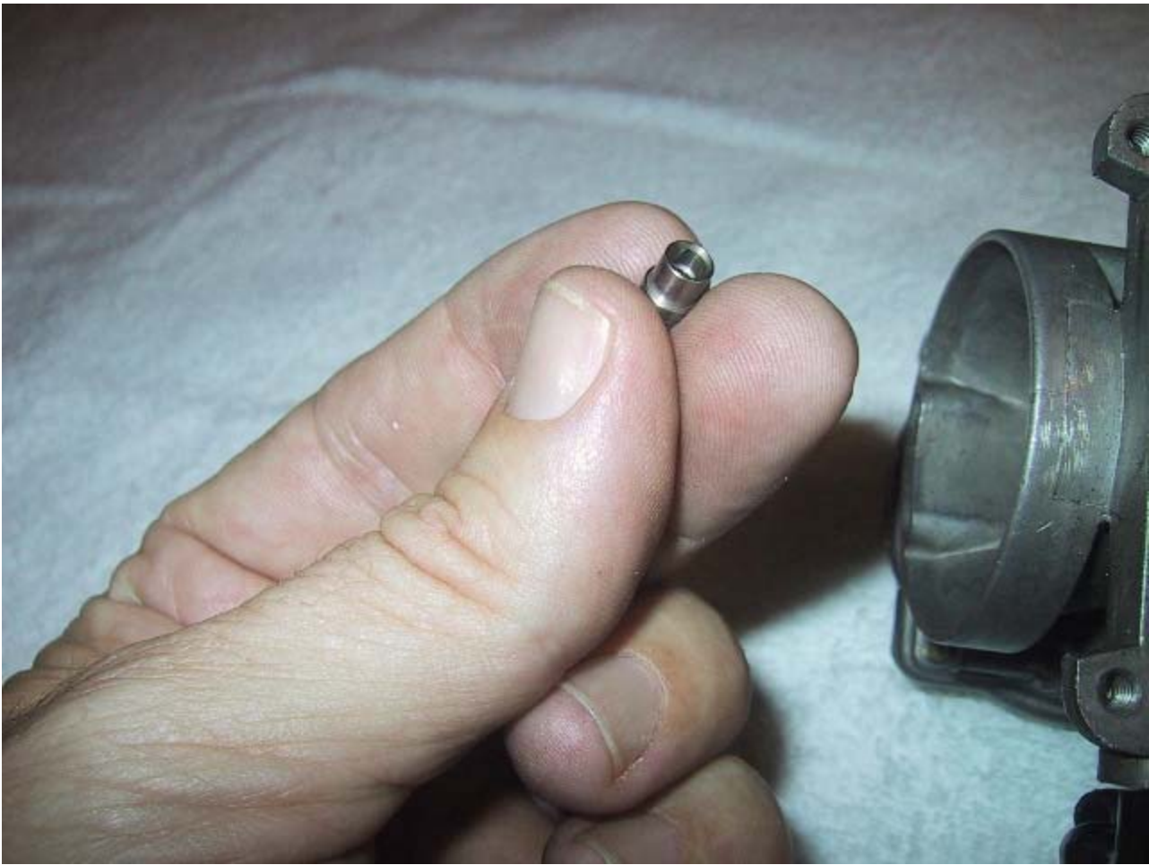
There are two distinct ends to the needle jet. This end goes in first.
