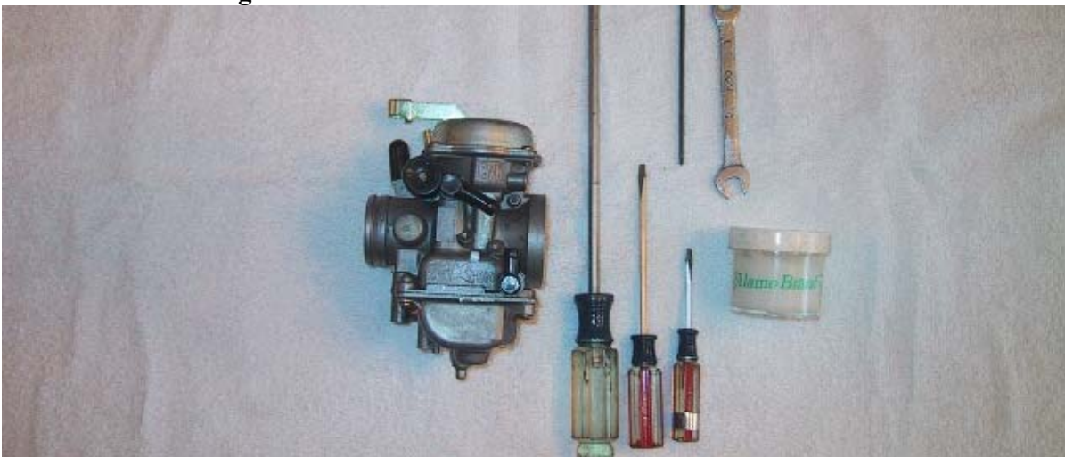
Tools needed to work on Keihin carb. Optional Pin gage set show below is available from Terry Crawford Ural.
