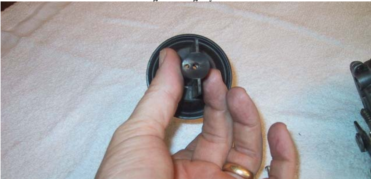
A little difficult to see in this picture...but the slide is off set and only goes into the carb body one way...don't force it...it should drop right in.
