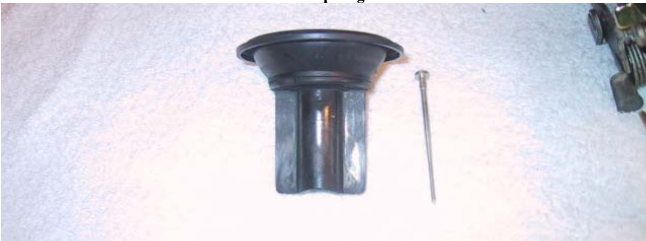
Caution again...the needle is not secured and can fall out if slide is inverted. If the needle or diaphragm gets damaged you are hosed.
