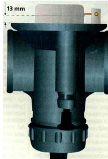
Adjust as necessary by bending the float support (#37 in Figure 1). Reinstall.
