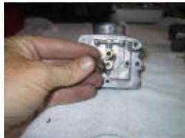
...remove the idle jet/tube and spacer gasket.
