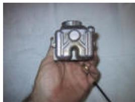
Bottom of the float bowl. There is no provision for a bowl drain unlike the Keihin carbs. To clean the bowl you must remove it.
