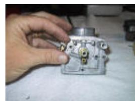
The seat threads are sealed with a small amount of thread compound. You should use some upon reassembly.
