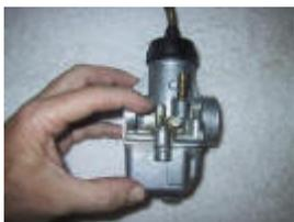
Index finger is pointing at tickler. This is used to prime the carbs for starting under normal conditions...
