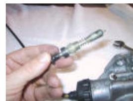
...and pull it free. It can be further disassemble by pulling the spring back and sliding the shaft out...but why?
