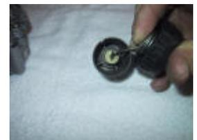
...which lets you disengage the throttle cable ferrule...
