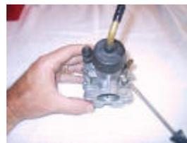
To begin disassembly, remove the float bowl retaining screws with the 3/16 's flat blade screwdriver.
