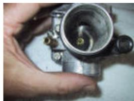
The alignment tooth is visible at 3 o'clock. Don't get the left and right slides mixed up as they are not interchangeable.
