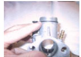
Note condition of O-ring and replace if needed. A little silicone grease keeps the O-ring in good condition.
