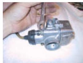
If you need to remove the choke mechanism, use a 13mm wrench to loosen the nut...
