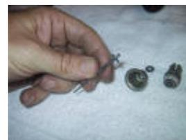
Ready to reinstall. The needle retaining nut threads can use some thread compound to keep it from vibrating loose.
