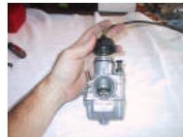
To get at the slide and needle, unscrew the plastic cap.
