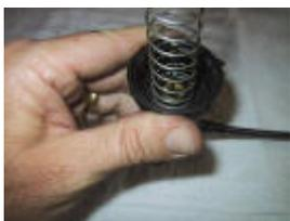
When putting the cap on make sure the spring goes inside the fingers inside the cap.
