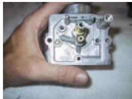
When reassembling the air tube. Make sure the flat of the nut is facing the idle jet gasket. If a point of the nut is facing it, you may cross thread the idle jet.
