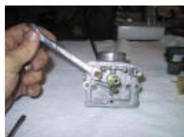
Use the 8mm wrench to remove the float needle seat.
