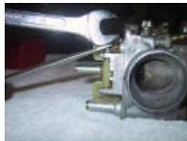
After inserting the float hinge pin, strike the splined end lightly with the blade screwdriver and wrench to seat it.
