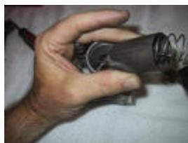
Make sure you line the slot up for the alignment tooth inside the carb body. It is easy to bummer the tooth if you are ham fisted.
