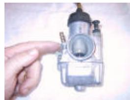
Air screw (not a mixture screw). Factory setting is 1.5 turns CCW from gently seated.
