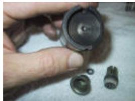
The needle is held in the slide by a ball bearing keeper see in the hole.
