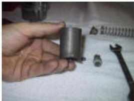
Use finger tip pressure on the tip of the needle to lift it up through the slide.
