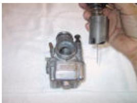
The throttle cable, cap spring, slide and needle come out as a unit. The cut out on the slide is for the idle adjustment screw.
