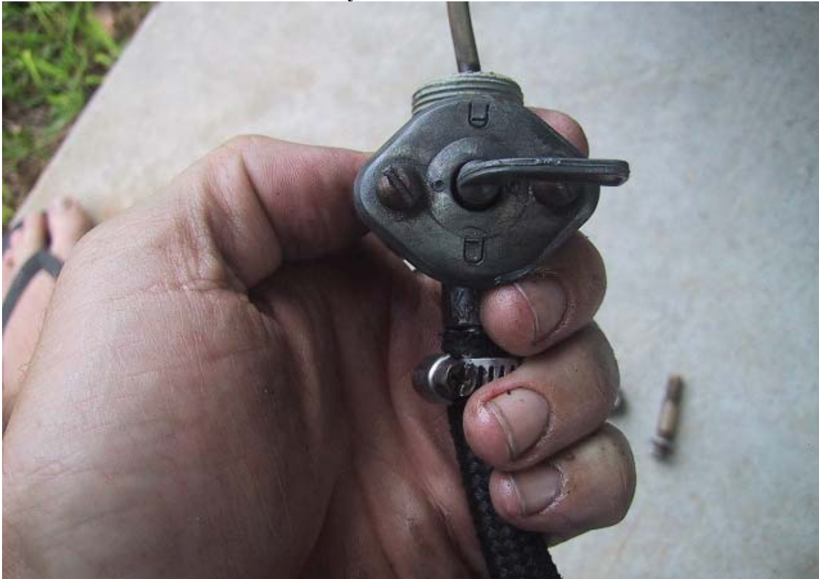
Just a shot of the face plate with the lever in the "Off" position. The upper symbol is for "Reserve" the lower is for "Main". The symbols depict the fuel level.
