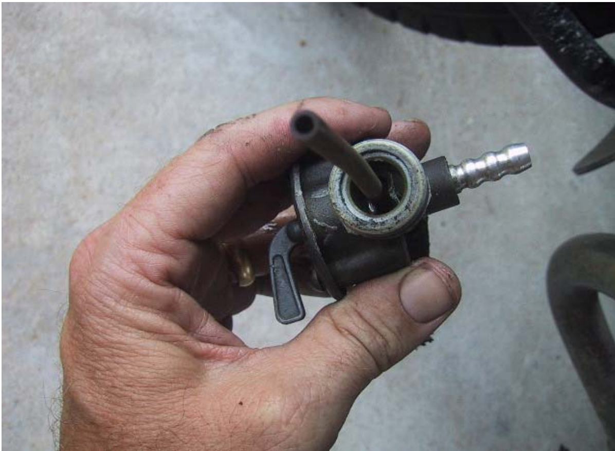
Just behind the stand tube is the flow hole for the "reserve" lever position. Lousy picture as it is almost not visible. In real life it is easy to see.
