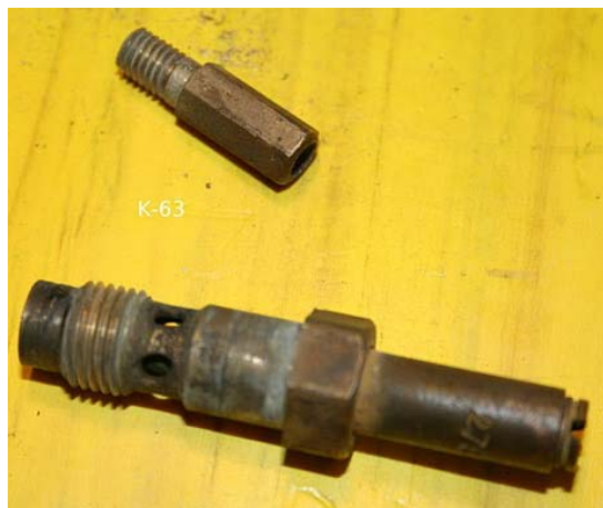
K-63 Idle Jet (above) and Main Jet Assembly (below)
