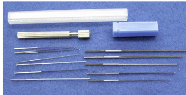
Set of 12 Jet Reamers with Holder for Jets with Bores from 0.6 to 2 mm Vendor Part #: S7005 Perfect for fine-tuning carburetors. List Price: 19.99€ (www.ural-zentrale.de)
