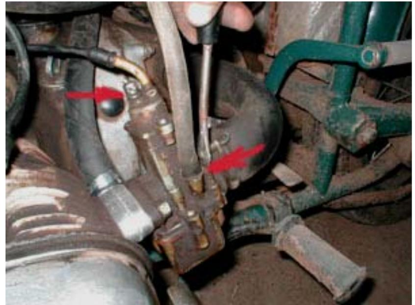
**Step10. When you mount both collectors and start engine, it will run a bit faster. You must re-adjust (lower) the idle screw - see red cursors.**
