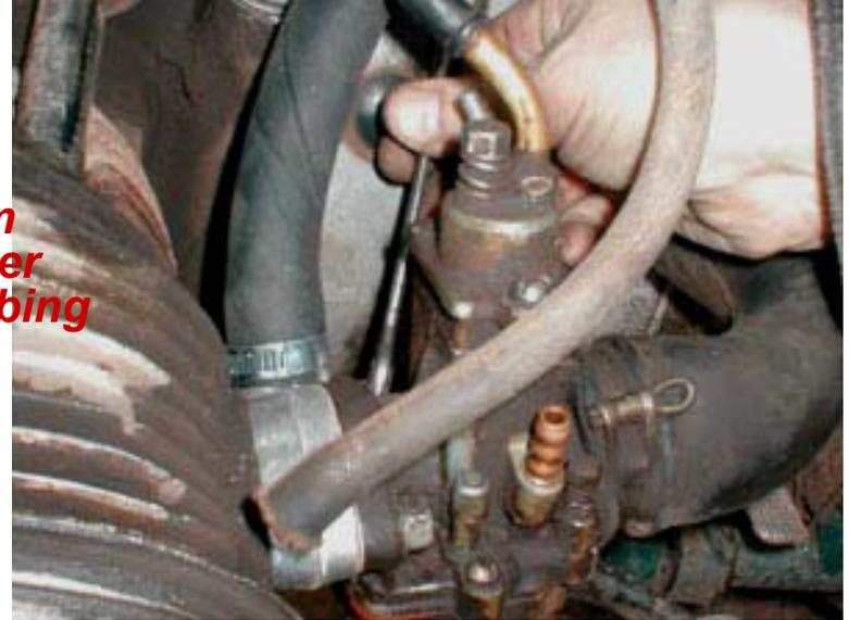
**Step 8. Mount carburetor onto collector.**
