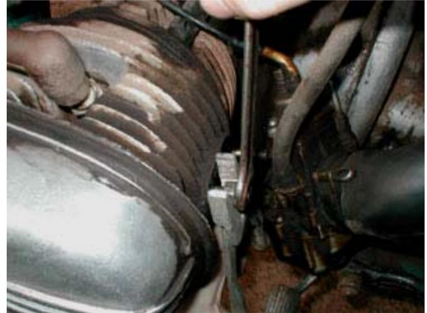
**Step 2. Lock two nuts (jam-nuts) on stud using two spanners (wrenches).**
