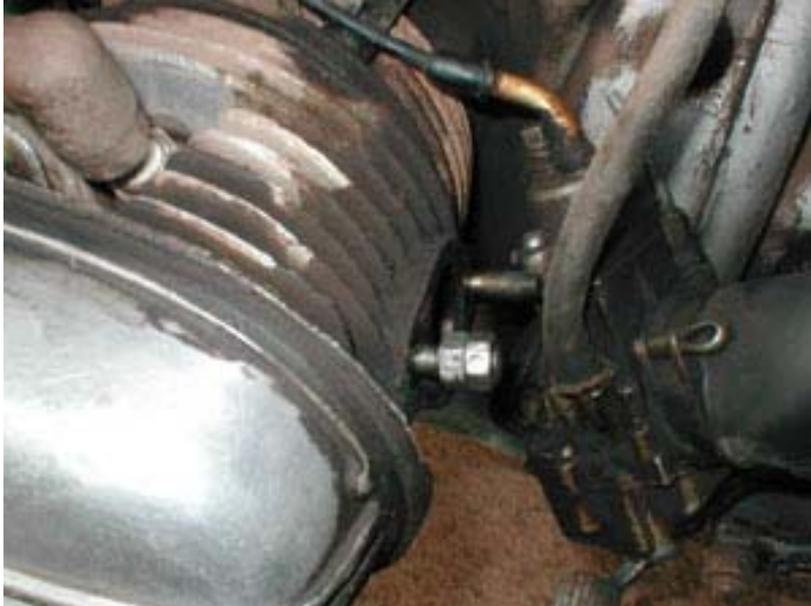
**Step 3. When you lock nuts, you can remove the old short studs.**
