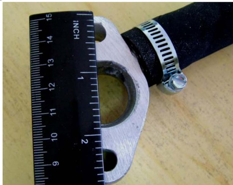
**Note: The mounting hole spacing may not be adequate, as imported bikes have a slightly greater spacing, and must be ovaled to fit.**
