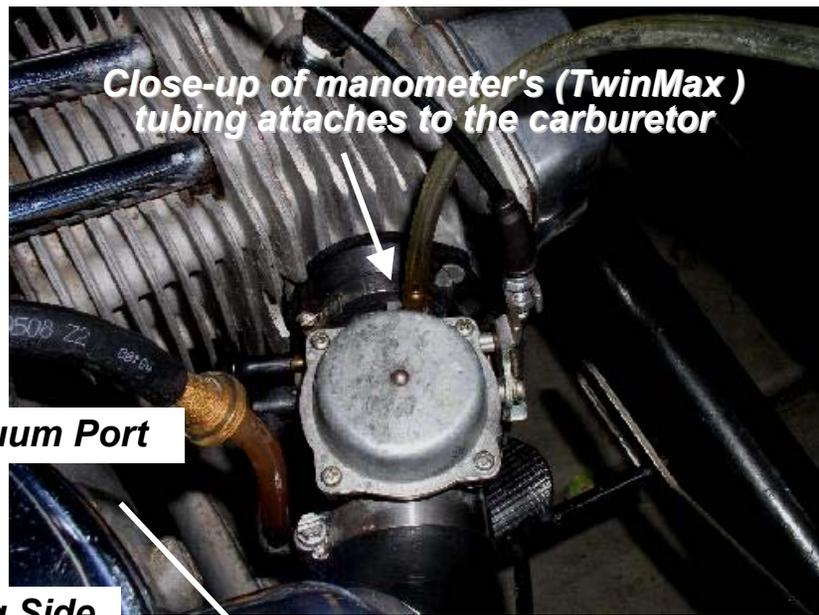
Close-up of manometer's (TwinMax) tubing attaches to the carburetor
