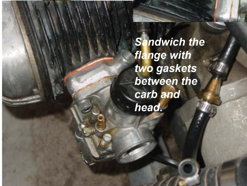
Sandwich the flange with two gaskets between the carb and head.
